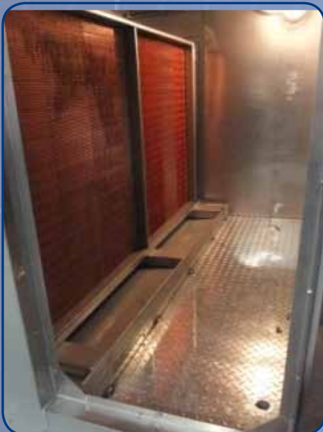
Drains, welded floors, water dams and wash down liner allow the inside to be cleaned with a hose
