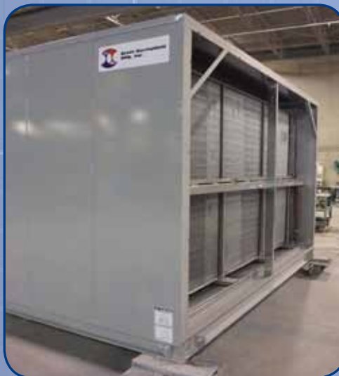
Structural angle split frame design assures rapid and precise assembly of multiple piece air handlers
