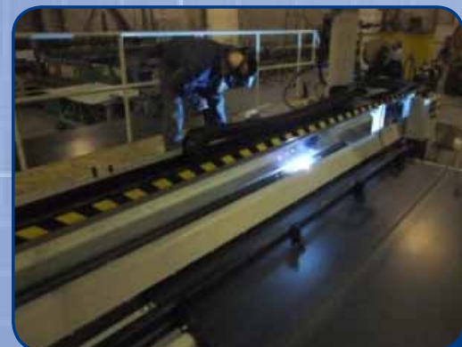
Fully welded floor seam prevents water or air leakage through the base
