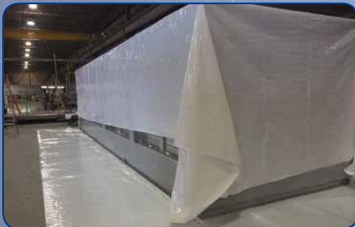
Every unit is shrink wrapped for delivery to prevent water damage to insulation that could lead to mold and IAQ issues
